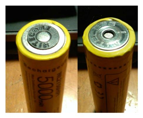
They need to access power on *both* ends of the cell. They've done to Olight trick on the top left image) by surrounding the (+) in the middle with a ring connected to (-). And on the tail end they have the big usual (–) base, and then thru a small hole you can poke in for the (+).
