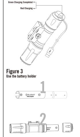
Install two CR123A batteries into the battery holder.
