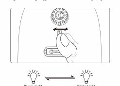
Stepless Brightness Control: Turn the knob clockwise to increase brightness. Turn the knob counterclockwise to decrease brightness.
