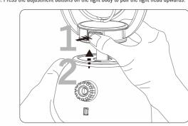
b. Hold and stretch the light head upwards to your desired height (the maximum height is 20cm).
